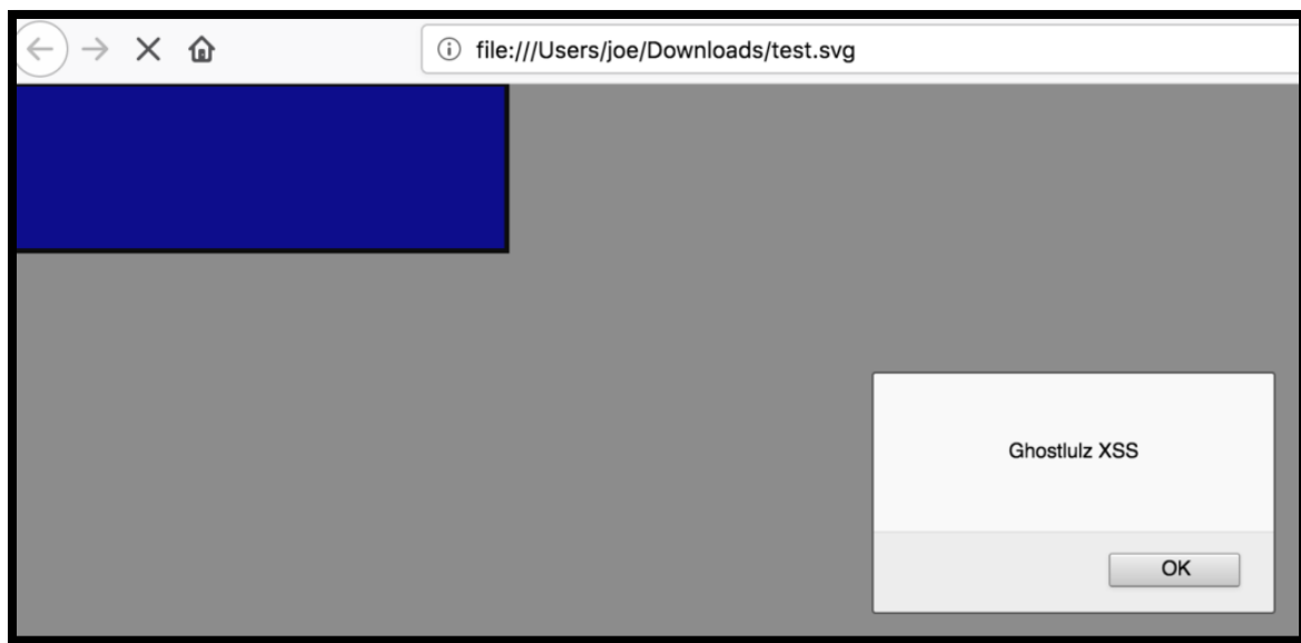
Figure 110: XSS payload triggering
